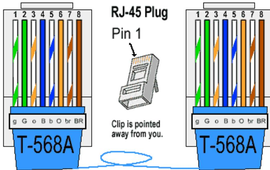
The T-568A standard was ratified in 1995 and has been updated in 2002 by T-568B which is supposed to be used in new network installations. You may find both standards in off-the-shelf Ethernet cables and it makes absolutely no functional difference in which you choose.
