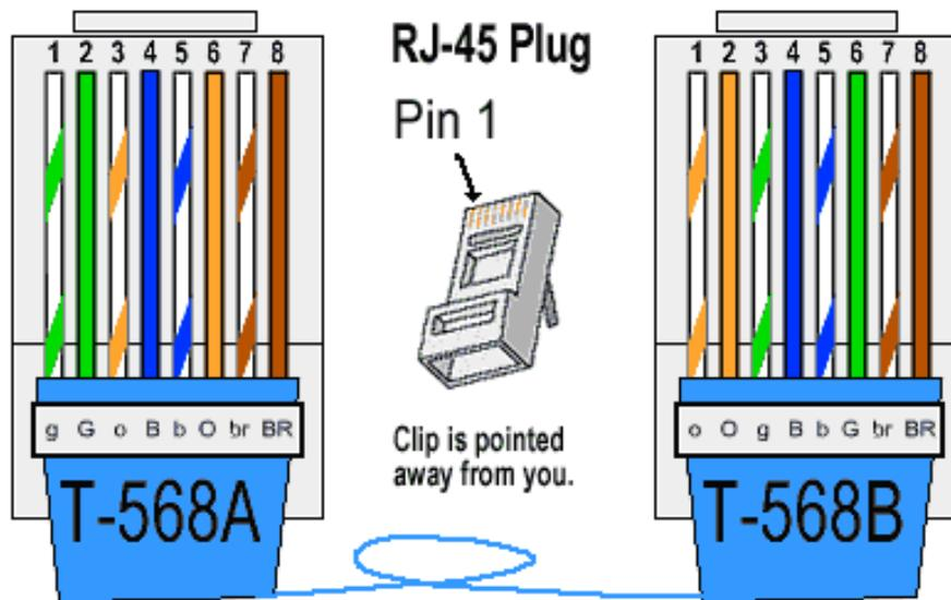
A good way of remembering how to wire a Crossover Ethernet cable is to wire one end using the T-568A standard and the other end using the T-568B standard. Another way of remembering the color coding is to simply switch the Green set of wires in place with the Orange set of wires. Specifically, switch the solid Green (G) with the solid Orange, and switch the green/white with the orange/white.
